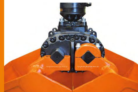
Remove connecting pieces one after another
